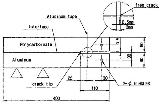
**Fig. 5** Configuration of test specimen
