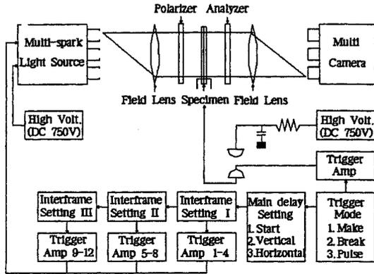
**Fig. 2** Block diagram of photoelasticity experimental setup
