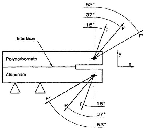
Fig. 6 Various mixtures of applied loads
