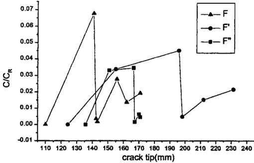
Fig. 11 Crack propagating velocities ( $C/C_R$ ) vs. location of crack tip ( $C$ : crack propagating velocities  $C_R$ : Rayleigh wave velocity of polycarbonate)
