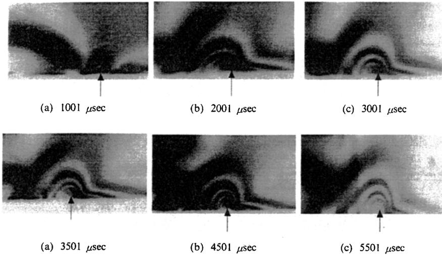
**Fig. 9** Dynamic isochromatic fringe patterns in polycarbonate for a crack dynamically propagating along the interface by initial load  $F'$  (crack runs left to right, scale: 4/1) ( $\mu\text{sec}$ =time after break,  $\longrightarrow$ : propagating crack tip location)
