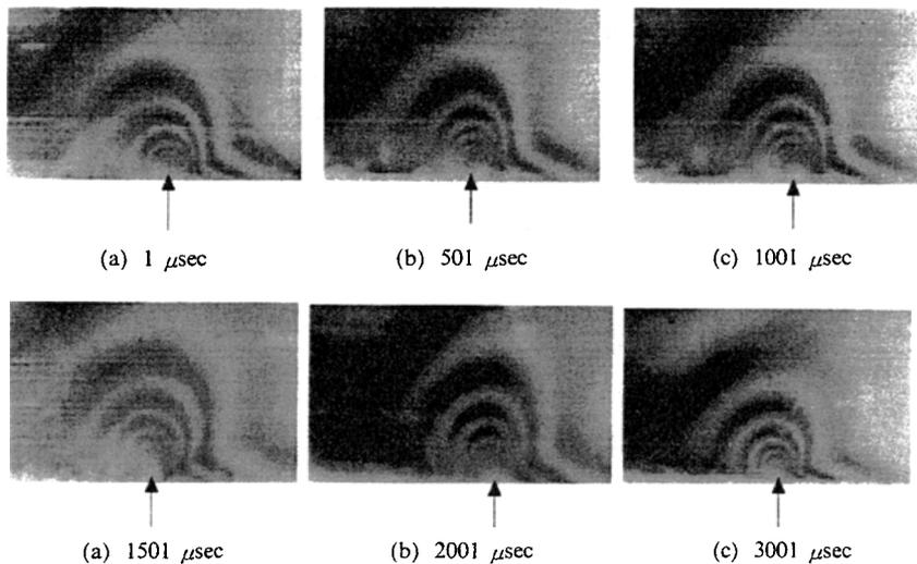
Fig. 8 Dynamic isochromatic fringe patterns in polycarbonate for a crack dynamically propagating along the interface by initial load F (crack runs left to right, scale: 4/1) ( $\mu\text{sec}$ =time after break,  $\longrightarrow$ : propagating crack tip location)
